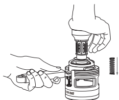
Impact pressure tamping (when there is sound feedback, it indicates that the tamping has been completed)
