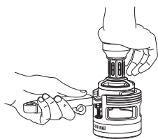
Adaptive height (maximum size of tamping is about 13mm)
